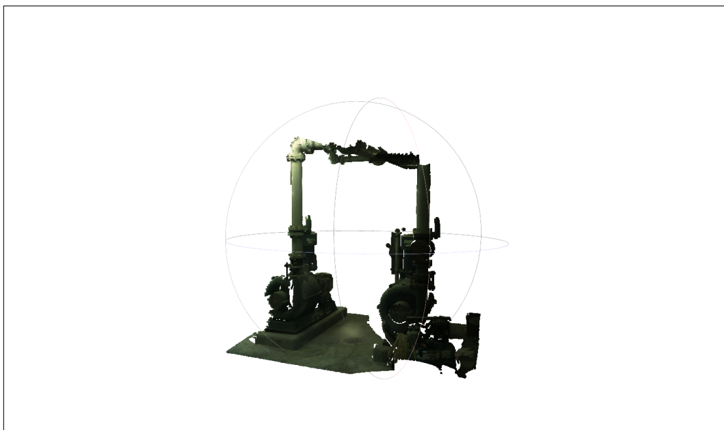
Figure 3.8: Pump . This is a single structured scan stored as cartesian and spherical points. Data includes intensity and RGB color. Screenshot captured in MeshLab 2021.07 during the test phase.
