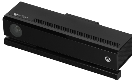
Figure 2.2: Xbox Kinect v2. The Kinect is an “active structured light” (active) 3D scanner, primarily thought to be used with the Xbox game console. Nowadays, Microsoft does not make any more game for the peripheral, but in the latest years a community of 3D hobbyists, that reevaluated the hardware, is born due to the device's lower cost.
