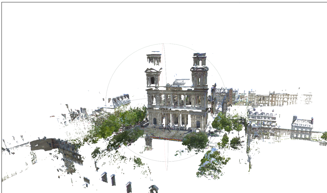
Figure 3.3: Trimble Data - Multiple Scans point cloud . This scene was scanned in Paris using a Trimble TX8 for project Terra Mobilita. Color has been captured with a Nikon 7100 using a fish eye Sigma 10 mm. Colorization and export to e57 has been done using Trimble RealWorks 8.1. The project contains one multi-station file (5 scans down-sampled at 50 mm going down from 650 M point to 8 M point) and two files containing gridded scans (down-sampled from 120 M point to 2 M point each). Gridded files are stored as spherical coordinates, and non-gridded ones use XYZ. Screenshot captured in MeshLab 2021.07 during the test phase.
